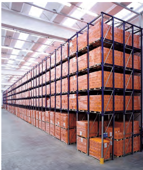
Figura 1-2: Scaffalatura porta pallet ad accumulo (Drive In, Drive Through)
